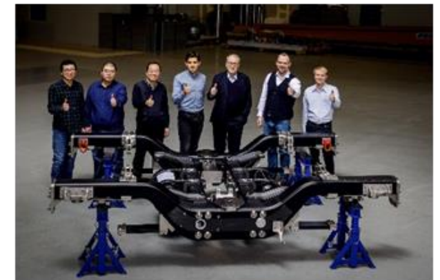
CG Rail – Lightweight CFRP-Bogie-Frame fully made of carbon-fiber reinforced plastic (CFRP) and offers a weight reduction of nearly 50 %
